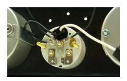
STEP 7: Connect the black ground wires from the lamp pigtails to the center ground studs of each smaller gauges as shown.
