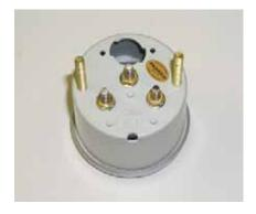
STEP 1: There are 4 small gauges. This is a photo of the bare gauge. Remove the 3 nuts and lock washers.
