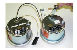
STEP 5: Install mounting clips on all gauges.
