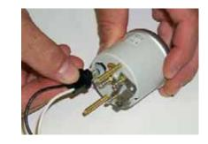
STEP 4: Install appropriate lamp socket pigtails into the speedometer & tachometer.
