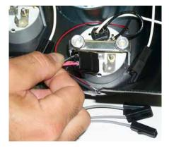
STEP 9: Plug in gauge connections using supplied connectors. Plug in connectors in the order shown below. Typical plug-in shown in picture.
